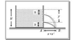
*i.e.*, the range will be same if the orifice is at a depth h or (H - h) below the free surface. Now as the distance (H - h) from top means H - (H - h) = h from the bottom, so the range is same for liquid coming out of holes at same distance below the top and above the bottom.
